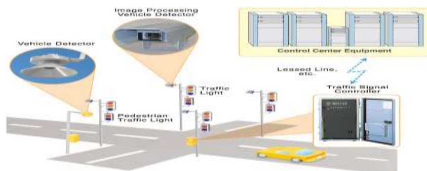
Figure 2: Smart Traffic Signal Control System Architecture
